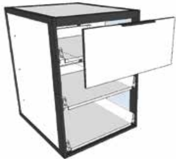
FIG. 19 To fit the drawer front to the drawer base, pull the base forward and place your palm in drawer base to hold push and click the drawer front into position.
